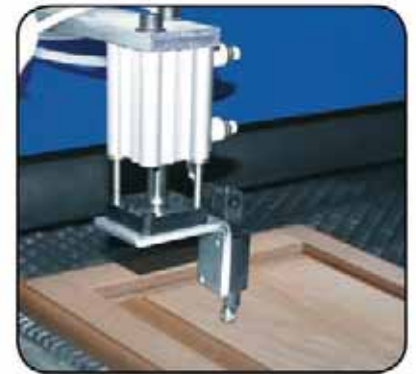
AUTOSSET (optional) - automatic thickness measuring of workpieces.
