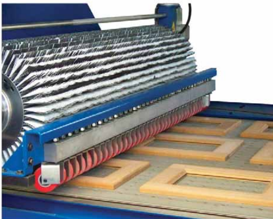
The F brush can be equipped with spring-loaded pressure rollers (optional) with tilting of the pieces that guarantee a seal optimal in all working conditions.
