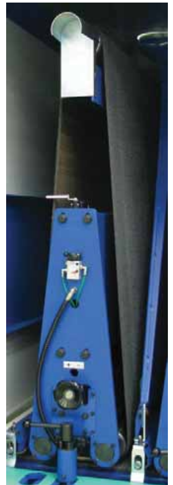
CA 16 - contact actuators pitch of 16 mm between sections
