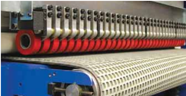
DB - Definition Barrier to detect size and form of panels to process with sectioned pads
