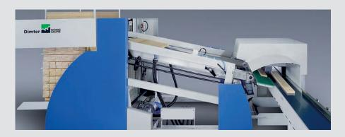
For the clear identification of the pieces after the cutting, inkjet or label printers are used.
