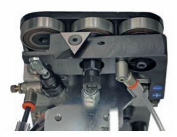
The **Glue Scraper** removes excess glue from the top and underside of the panel. This is the only model on the market fitted with 4 pneumatic cylinders for a top quality finish.
