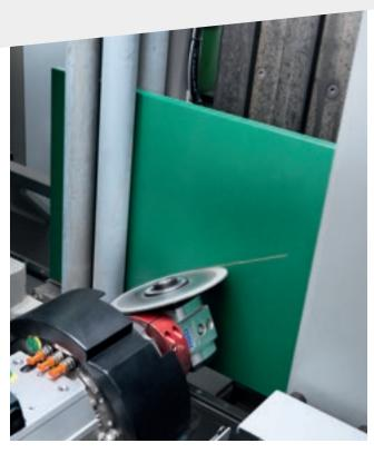
Cutting machine with integrated C-axis (optional).
