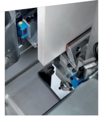
The **laser scanner** system that detects the start and the end of the panel enables the machine to compensate dimensional errors, correcting the panel's X dimensions.
