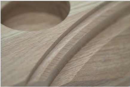
Application examples: the t3-System cutter creates chip-free jointing and hemming surfaces.
