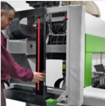
New hood with openable Plexiglass front door, for ease of operation.
