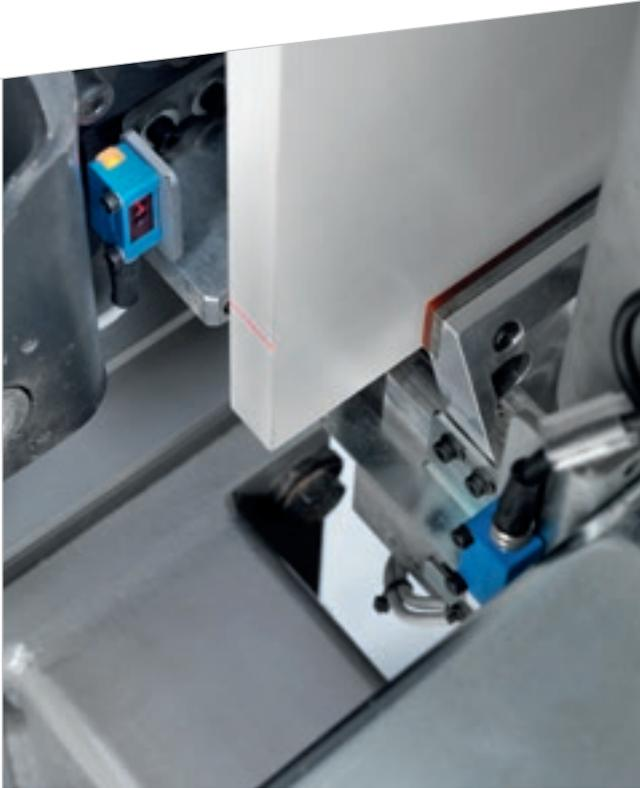
The **laser scanner** system that detects the start and the end of the panel enables the machine to compensate dimensional errors, correcting the panel's X dimensions.
