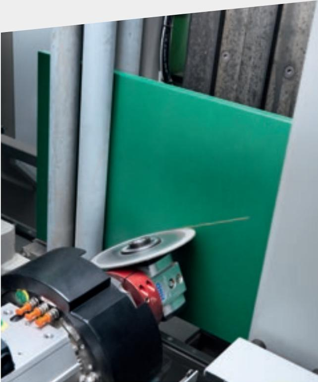
Cutting machine with integrated C-axis (optional).
