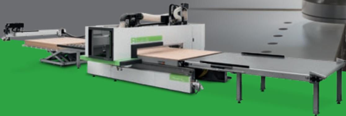
Rover A FT is the new high-performance machining centre for Nesting operations. Compact and efficient, with a gantry structure, the Rover A FT offers top-of-the-range technology and guarantees optimum precision in every machining operation.
