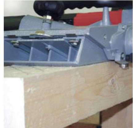
With guide rollers - for maximum utilisation of the planing width.
