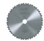
TCT saw blade 250 x 1.8/2.8 x 30 mm (9 13/16 in.), 24 teeth, AT, for ripping cuts
