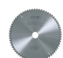
TCT saw blade 250 x 1.8/2.8 x 30 mm (9 13/16 in.), FT/TT, 68 teeth, for plastic and aluminium profiles
