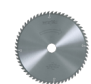
TCT saw blade 250 x 1.8/2.8 x 30 mm (9 13/16 in.), AT, 60 teeth, for fine cuts
