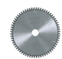
TCT saw blade 225 x 1.8/2.5 x 30 mm (8 7/8 in.), FT/TT, 68 teeth, for plastic and aluminium profiles
