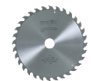
TCT saw blade 225 x 1.8/2.5 x 30 mm (8 7/8 in.), AT, 32 teeth, for universal use
