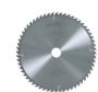
TCT saw blade 250 x 1.8/2.8 x 30 mm (9 13/16 in.), AT, 60 teeth, for fine cuts
