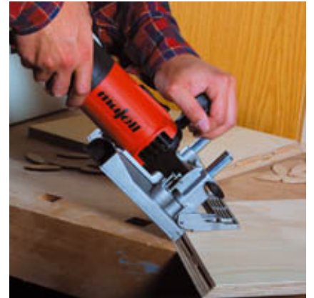
Mitred joints with the LNF 20.
