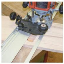
Available as a special accessory, the router guide device for cutting housings in staircase strings can execute all cuts up to 640 x 60 mm.
