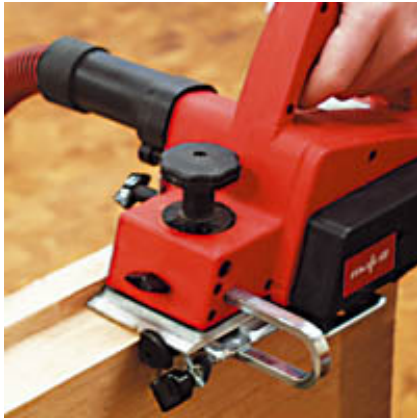
Re-rebating of a door with the MHU 82.
