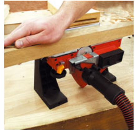
Chips are simply removed by suction.
