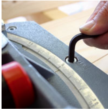
The slot mortiser can be tilted through 45° in either direction.
