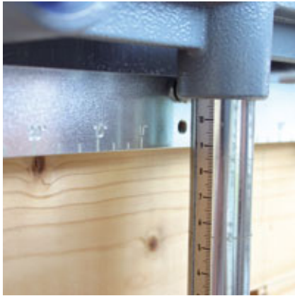
The vertical edge spacing is set exactly by way of a scale.
