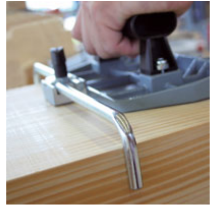
The clamp is continuously adjustable for series production purposes.
