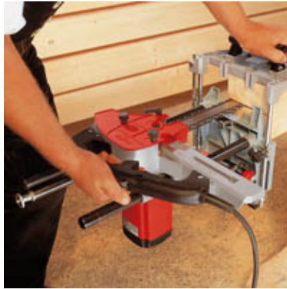
Mortising direction with the SG 230 - vertical and horizontal.
