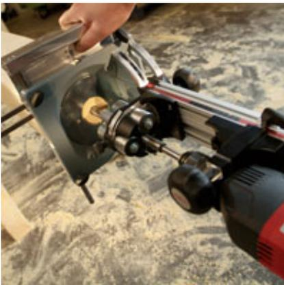
The parallel fence, typically used for end grain drilling, is an ideal accessory to the face edge stop for series production purposes.
