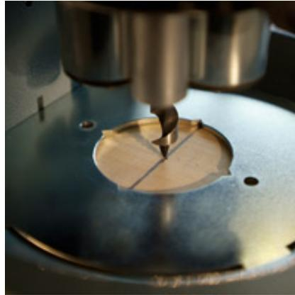
Notches to facilitate marking enable you to position the drill with great accuracy. Even when working at an angle, the drill tip always serves as the pivot axis.
