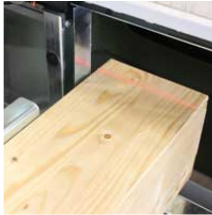
Laser technology allows positioning of the workpiece after marking.
