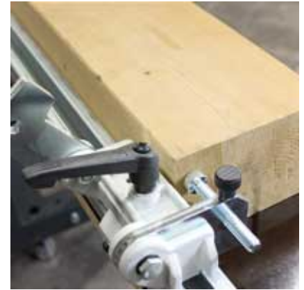
The 3 m (9.8 ft) long support profile with mm scale and length stop allows precise positioning of the workpieces.
