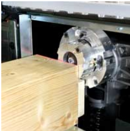
Straight and angled tenons are executed in a single work cycle as the control permits machining on 4 sides. This also allows all-round chamfering of the tenons.
