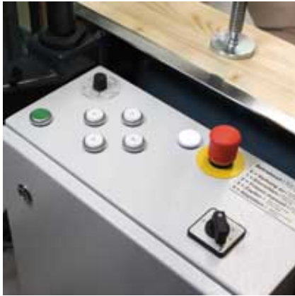
Clear, transparent layout – the controls of the ZAF 250 Vario for automatic or manual operation.
