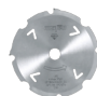
Saw blade Dia 160 x 2.4/3.0 x 20 mm (6 5/16 in.) / 4 flat/trapezoidal teeth for cement-bonded materials
