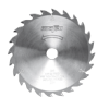
TCT saw blade 160 x 1.2/1.8 x 20 mm (6 5/16 in.), AT, 24 teeth, for universal use in wood
