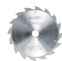
TCT saw blade 160 x 1.2/1.8 x 20 mm (6 5/16 in.), AT, 16 teeth, for rip cuts in wood
