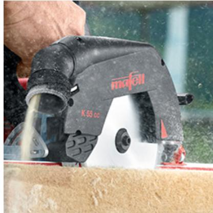
The chips are carried away so efficiently that the vacuum channel cannot become blocked. Users enjoy this crucial benefit when executing plunge cuts in the direction of the fibers as well.
