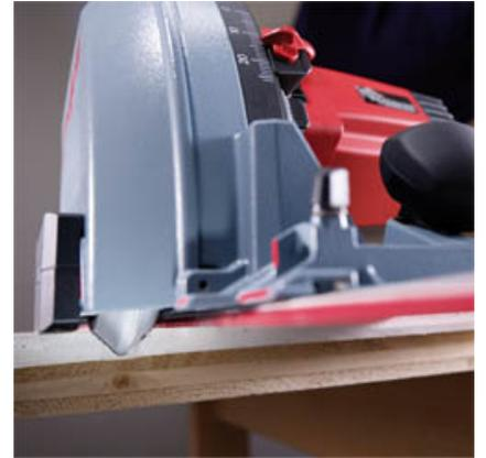
The MF-GF 90 cuts 90° V-grooves with very little dust; by gluing the cut faces, sturdy corner paneling is produced in just a few steps.
