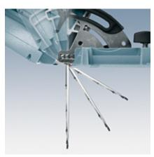
The tilt range of 0° – 60° enables extreme bevel cuts.
