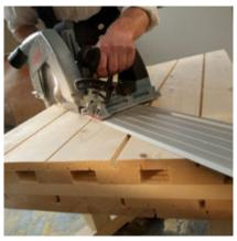
To enhance precision, the MKS 130 Ec can be used together with a guide rail.
