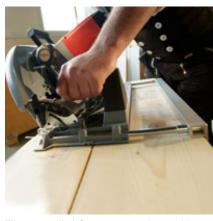
The parallel fence, together with the ample reserve power of the new, high-performance CUprex motor, are further guarantors of precise guidance and clean cuts.
