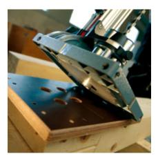
For series drilling and hole patterns, the insertion plate can be replaced by a copying insert. Ideal when working with drilling templates.
