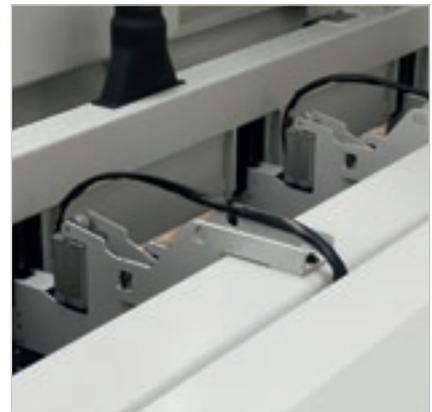
The consistent, controlled pressure on the book of panels to be cut is guaranteed by the **presser** with its single-element structure.
