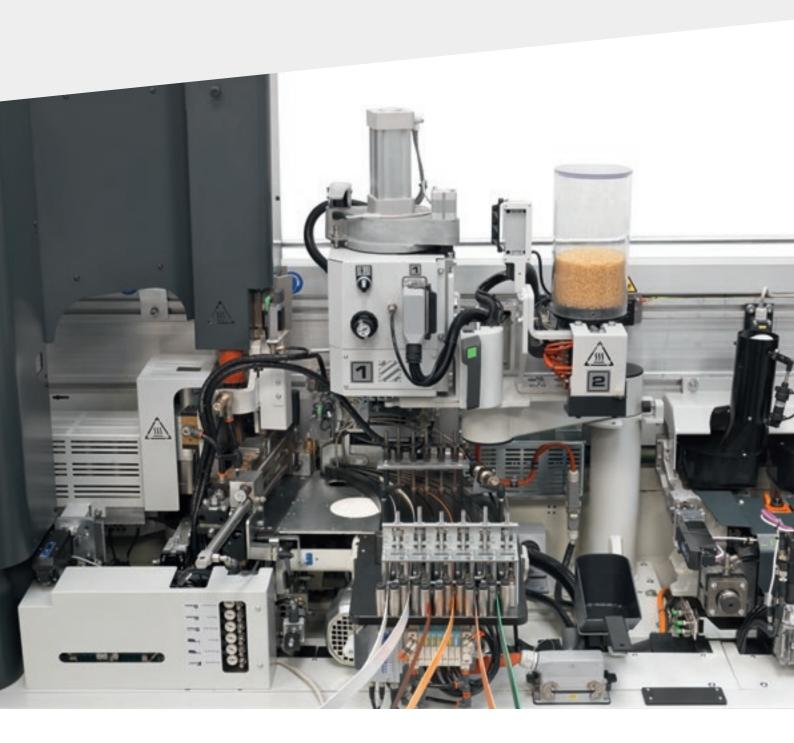
Thanks to the new gluing device designed for Stream A, the gluing unit can now house 2 pre-melters that can be alternated with just a few steps.
