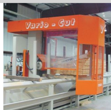
Any system length possible due to self-supporting rail guide
