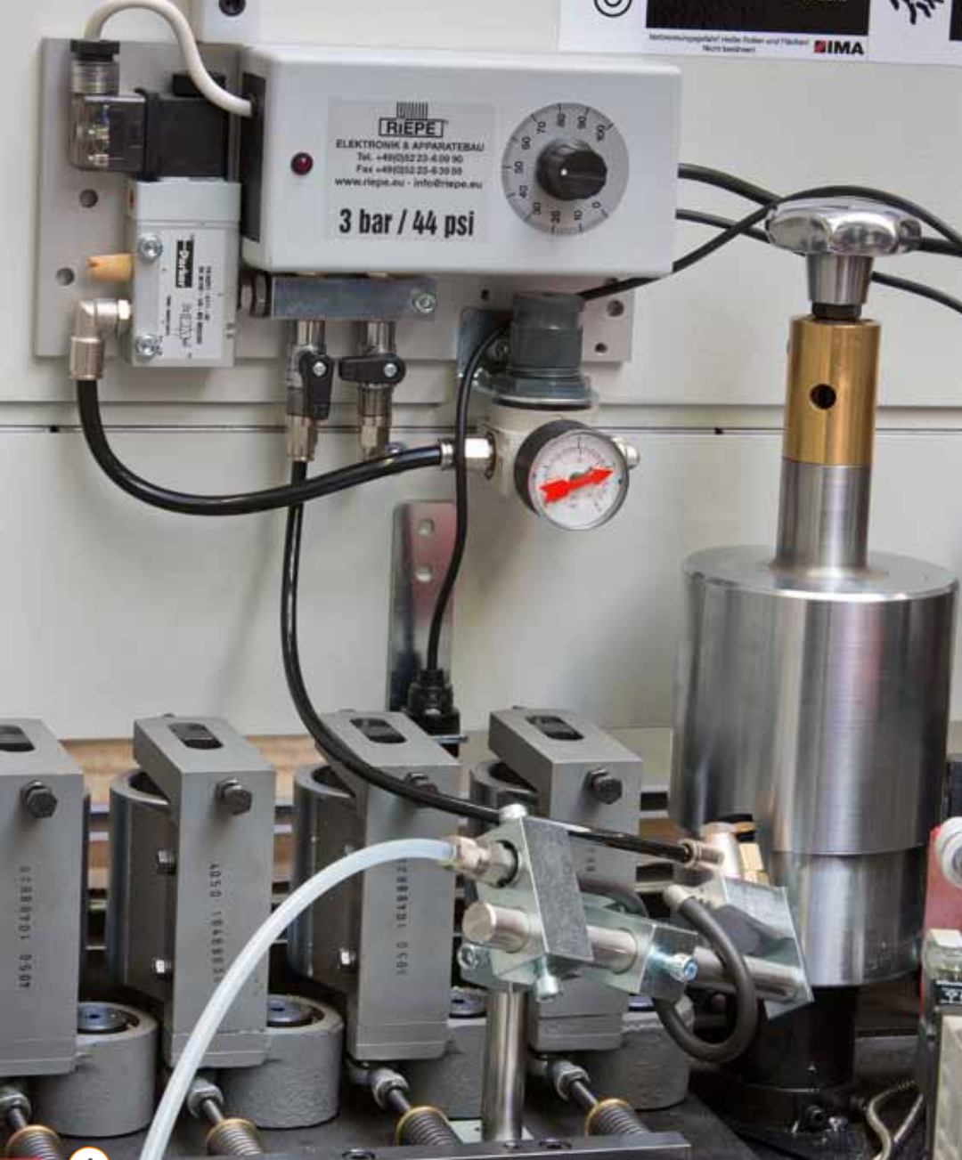
1 Installation example release agent spraying system for the pressure roller
