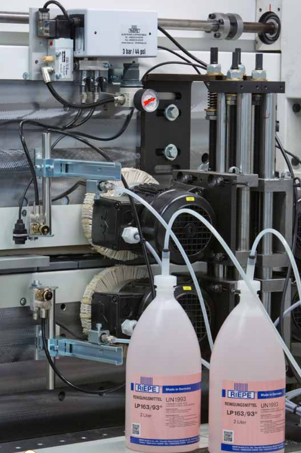
1 Installation example cleaning agent spraying system in front of the buffing wheels
