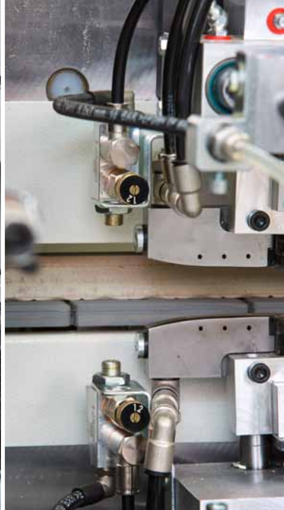
2 Installation example cleaning agent spraying system in front of the flat scraper
