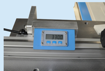
Digital read-out and one large swivelling back stop
