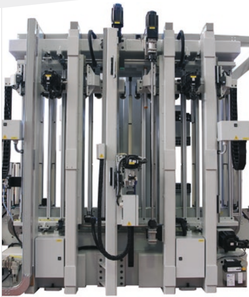
Unit for opposed boring, for completing the machining operations on the rear face of the panel.
