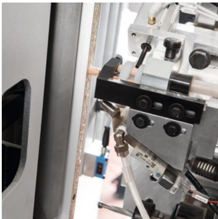
Unit for managing the boring operation and the insertion of glue and dowels.
