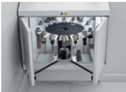
The machine can also be equipped with a rotating magazine (holding up to 16 tools) on the right-hand side to facilitate tooling operations.
