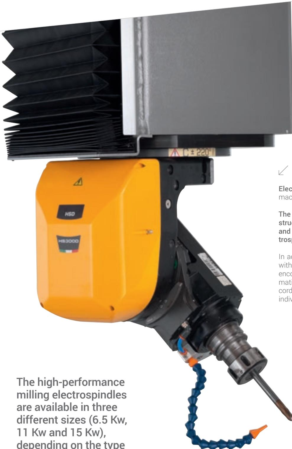
The high-performance milling electrospindles are available in three different sizes (6.5 Kw, 11 Kw and 15 Kw), depending on the type of machining operation required.
