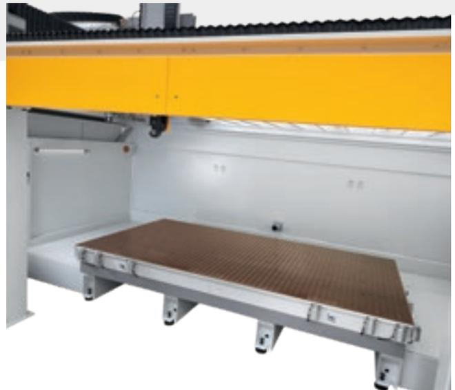
The grid surface allows the operator to insert the gasket in any configuration, creating a specific vacuum area. An internal chamber ensures the even distribution of the vacuum all over the work table.
