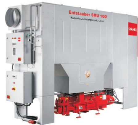
SMU 60 - 100 series with briquetting press
