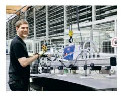
VacuMaster. With the ergonomic operator handle, the user maintains the required safety distance from the picked-up object and transports it to its destination safely, gently and without exerting force. Unlike the Jumbo, the VacuMaster only holds the workpieces. The lifting movement is performed by a chain hoist.
