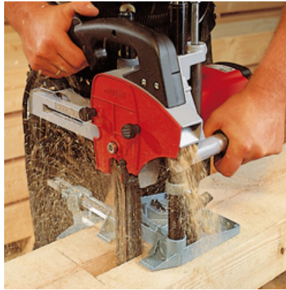
The LS 103 Ec with the guide support stand FG 150 for mortising depths of up to 140 mm.
