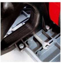
The tool for replacing knives is mounted directly on the machine.
