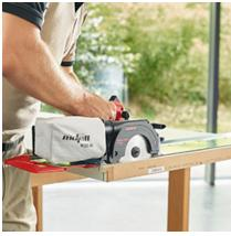
In combination with the roll-up Flexi-Guide FX 140, precise guided cuts up to 1.4 m (4.6 ft) long can be executed with consummate ease.
