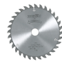
TCT saw blade 168 x 1,2/1,8 x 20 mm, Z 32, WZ, for fine sawing in wood
