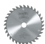
TCT saw blade 168 x 1,2/1,8 x 20 mm, Z 32, WZ, for fine sawing in wood
