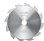
TCT saw blade 237 x 1.8/2.5 x 30 mm (9 5/16 in.), AT, 12 teeth for rip cuts in wood
