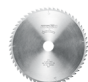
TCT saw blade 237 x 1.8/2.5 x 30 mm (9 5/16 in.), AT, 56 teeth for cross-cutting in wood
