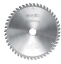
TCT saw blade 162 x 1.2/1.8 x 20 mm (6 3/8 in.), AT, 48 teeth, for universal use with board materials
