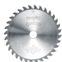
TCT saw blade 160 x 1.2/1.8 x 20 mm (6 5/16 in.) / AT, 32 teeth, for fine cuts in wood
