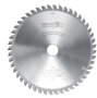
TCT saw blade 162 x 1.2/1.8 x 20 mm (6 3/8 in.), AT, 48 teeth, for universal use with board materials
