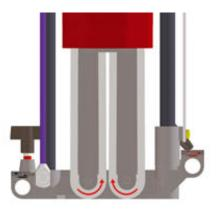
Two special mortising chains in opposite directions ensure tear-free work and optimum chip flow.
