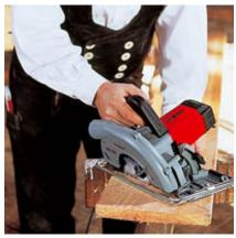
The angle can be set exactly and fixed on the scale between  $0^{\circ}$  and  $45^{\circ}$
