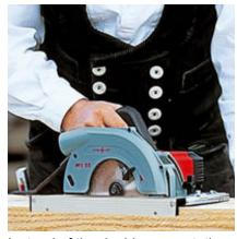
Instead of the double support, the MAFELL parallel guide fence can be used. This is available as an optional accessory.
