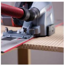
Three slots can be cut in one pass with the MF-SE 3. This quick and simple bending technique is applied to produce curved elements.
