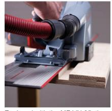
Equipped with the MF-VN 25, the multicutter can produce grooves for risers or service ducts efficiently and quickly.
