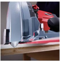
The MF-GF 90 cuts 90° V-grooves with very little dust; by gluing the cut faces, sturdy corner paneling is produced in just a few steps.
