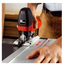
If exactly straight cuts are required, the P1 cc can be used in conjunction with the MAFELL F guide rail.
