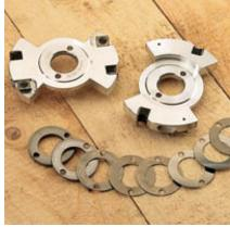
The width of the expanding grooving cutter is adjusted with a combination of different spacer rings.
