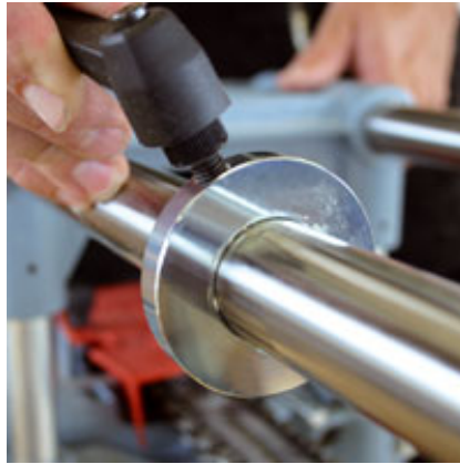
The cutting depth can be set exactly.
