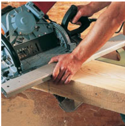
Ideal application e.g. for rafter cuts. The universal guide support as an optional accessory.
